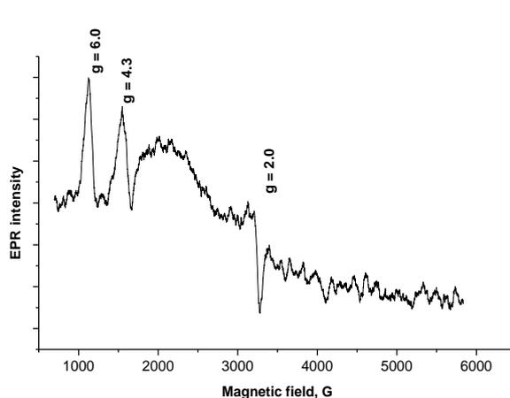
**Figure 4.** EPR spectrum of blood of Chernobyl clean up worker. (Documented dose in register 0.211 Gy.  $^{90}\text{Sr}/^{90}\text{Y}$  activity measured on teeth in 1997 - 80 Bq/g).
