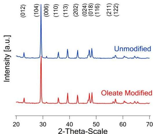
**Figure 1.** XRD patterns of the prepared calcium carbonates
