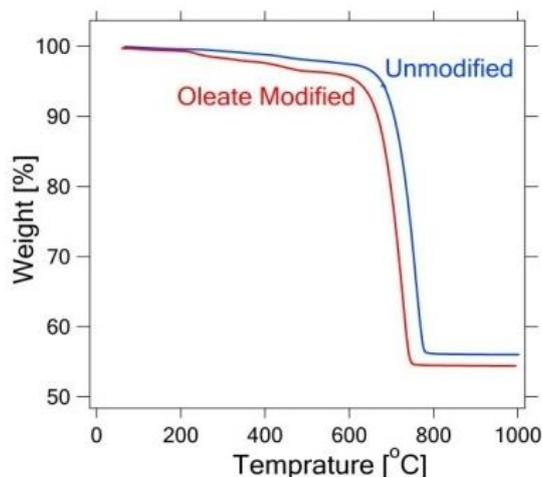
Figure 5. TGA curves of the prepared calcium carbonates
