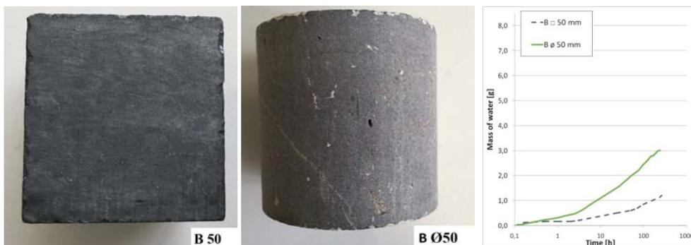
**Figure 4a.** Selected samples and their capillary absorptivity plots - basalt
