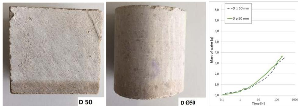
**Figure 3a.** Selected samples and their capillary absorptivity plots - limestone
