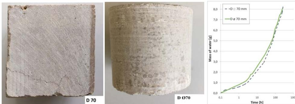
**Figure 3b.** Selected samples and their capillary absorptivity plots - limestone
