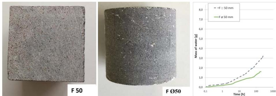
**Figure 4b.** Selected samples and their capillary absorability plots - limestone
