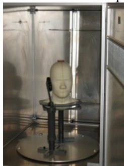
Figure 3. TRP measurement using a compact mode-stirred reverberation chamber. The TRP are measured for the same configurations (same frequency channel and use position) as those required for the SAR compliance of mobile phones.
