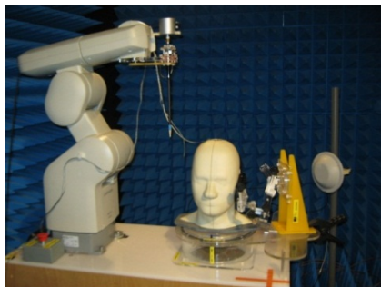
Figure 1. SAR measurement using a six-axis robot and the SAM phantom filled with tissue equivalent liquid. The SAR measurements are performed at the center frequency of a given band for four intended use positions of the mobile phone against the phantom. Two additional measurements are then performed at the two extreme frequencies of the band for the worst-case position.
