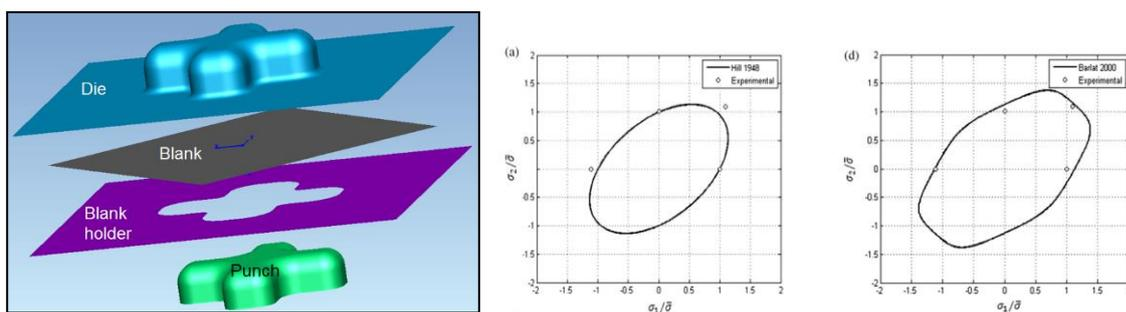
**Figure 5.** FE Model of the Cross Forming Using the PAM-STAMP (left), Hill 48 anisotropic yield function (middle) and Barlat 2000 anisotropic yield function for elevated temperatures (right).
