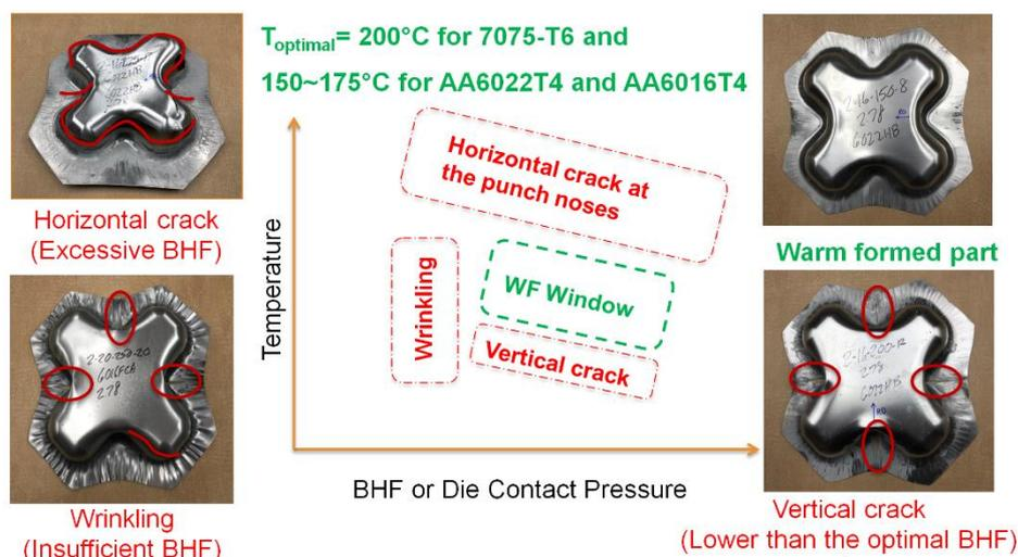
**Figure 3.** Warm Forming Process Window.
