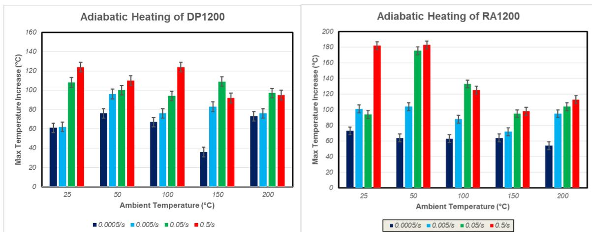
**Figure 3.** Maximum temperature increase on the DP1200 and RA1200 specimens.
