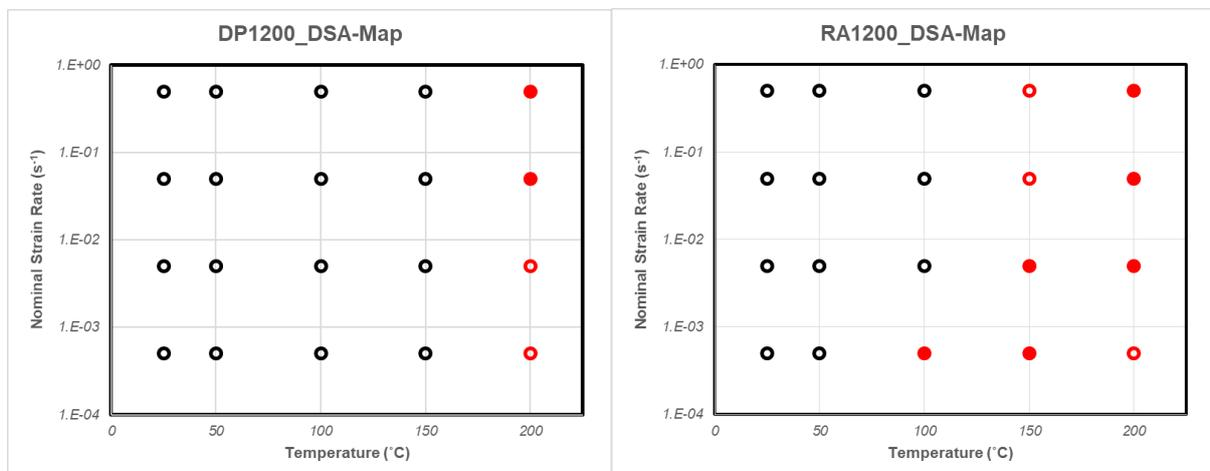
**Figure 5.** The DSA activation maps of DP1200 (left) and RA1200 (right): the black hollow circle shows the DSA-free conditions, the red hollow circle means the DSA region with only the negative strain rate
