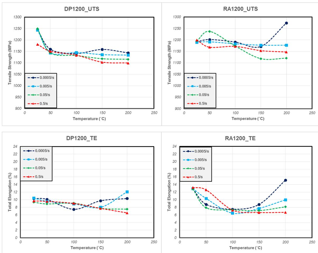
**Figure 6.** The DSA effects on the tensile properties of the DP1200 (left) and the RA1200 (right).
