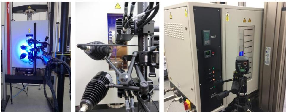
**Figure 1.** The experimental set-up including DIC and infrared camera.
