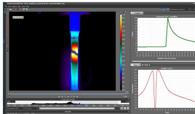
**Figure 2.** Thermographic measurements capturing the peak temperature.
