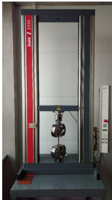
Figure 6. Test stand with installed specimen– Zwick Roell Z050.
