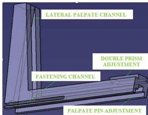
**Figure 8.** Mobile prism – constructive elements.
