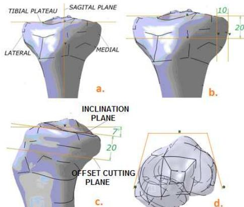
**Figure 5.** Geometrical references for HTO.
