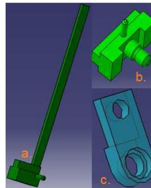
**Figure 9.** Palpate pin, slider part spigot, bush support plate.
