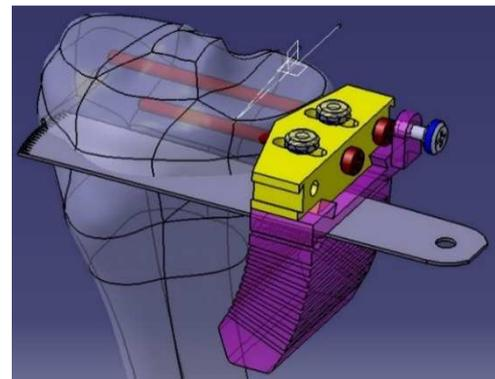
**Figure 14.** Device for closing High Tibial Osteotomy – manufacturing of the cuts.
