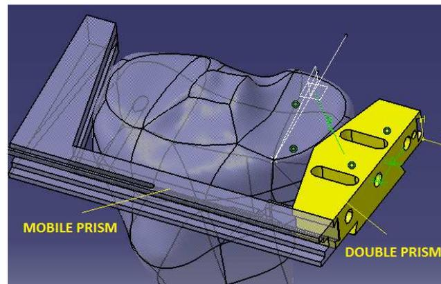
**Figure 6.** Fixation prisms elements.
