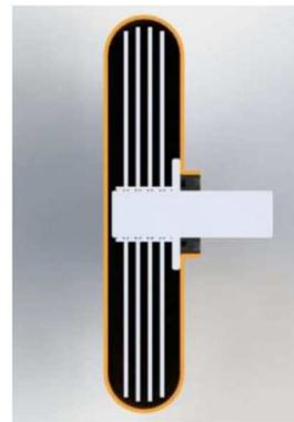
**Figure 2.** Cross section of bladeless centrifugal heart pump [16].
