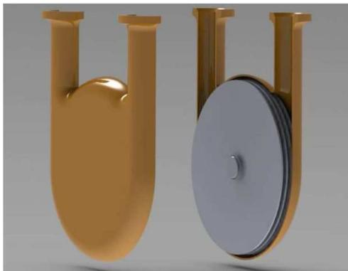
**Figure 1.** Geometrical model of bladeless centrifugal heart pump [16].
