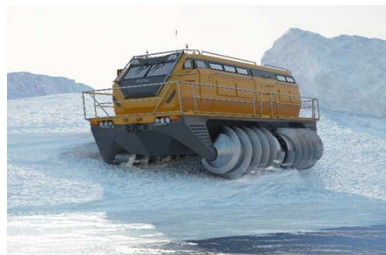
Figure 3. Residential vehicle based on unified rotary-screw platform.
