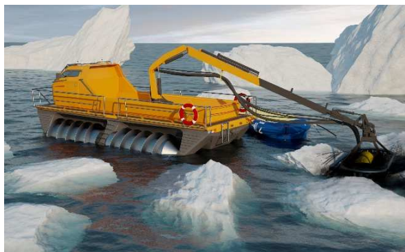
Figure 4. The unified platform with oil spill response equipment.
