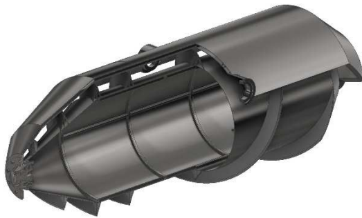
Figure 14. Computer 3D model of rotary-screw propeller.
