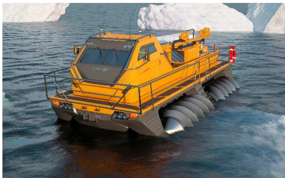
Figure 2. Unified rotary-screw platform with drilling rig.
