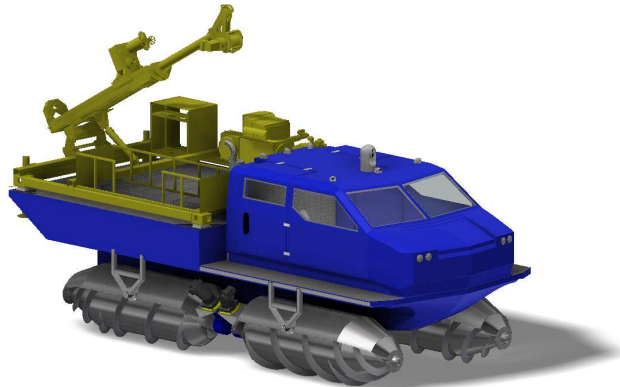
Figure 8. Computer 3D model of an experimental model with a small drilling rig.
