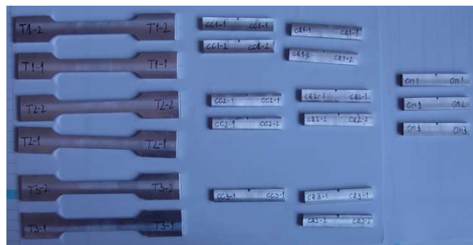
Figure 6. Tensile specimens and impact test specimens.
