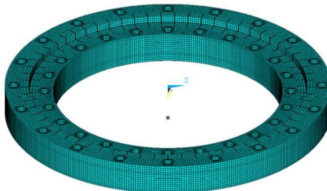
**Figure 5.** FEM model of slewing bearing.
