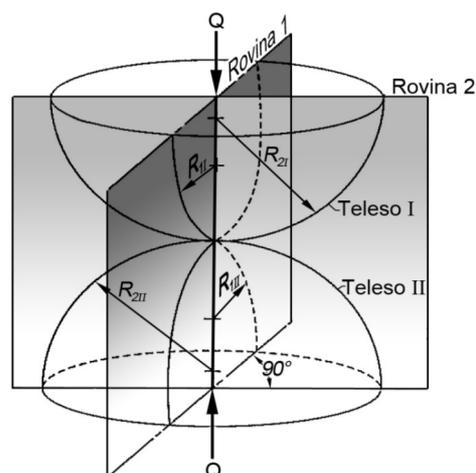
**Figure 2.** Radii of curvature located in main planes.
