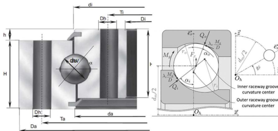
**Figure 4.** Geometrical parameters of the slewing bearing.
