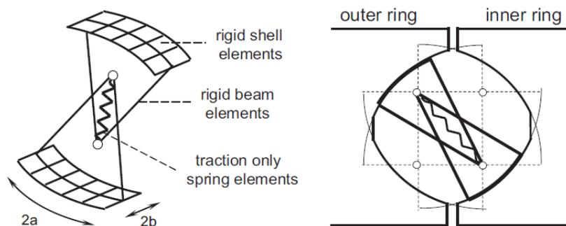
**Figure 6.** Schematic representation of the model for the ball and the ball raceway contact.
