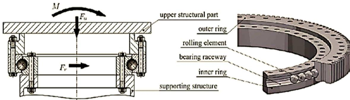
**Figure 1.** Typical arrangement of four contact point slewing bearing.
