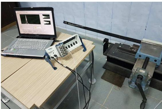
**Figure 8.** Experimental stand dedicated for natural frequency estimation of beams.
