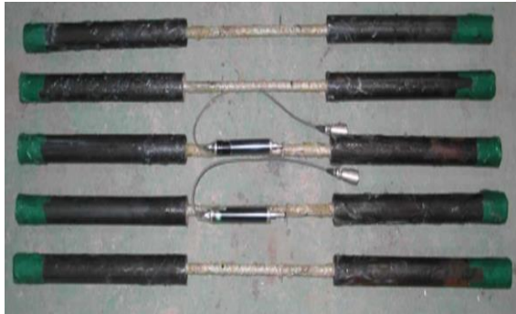
Figure 2. Specimens of FRP re-bars.
