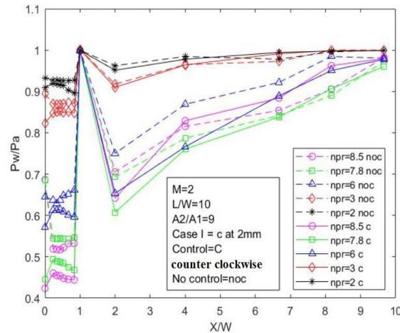
**Figure 8.** Flow development in the duct at different NPR for Case I
