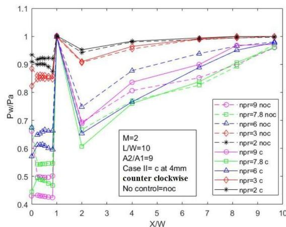
**Figure 9.** Flow development in the duct at different NPR for Case II
