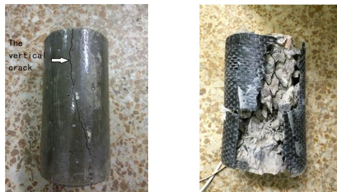
Figure 4. Failure models of columns
