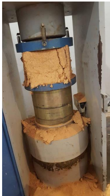
Figure 1. Compressive strength test setup. Figure 2. Flexural strength test setup.
