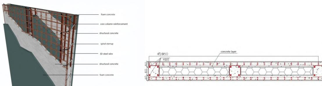
**Figure 1.** Section of the new fabricated sandwich panel.
