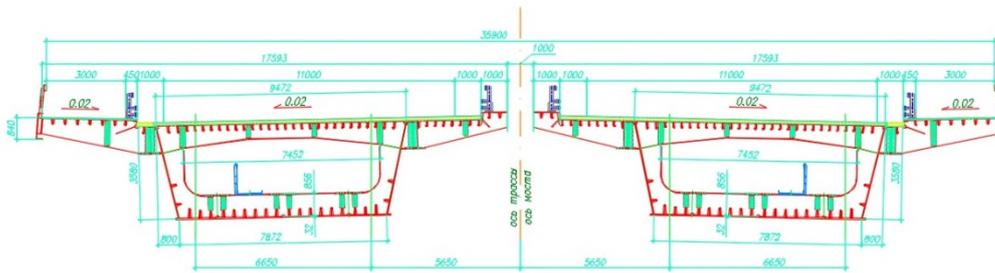
**Figure 1.** Cross-section of the bridge.
