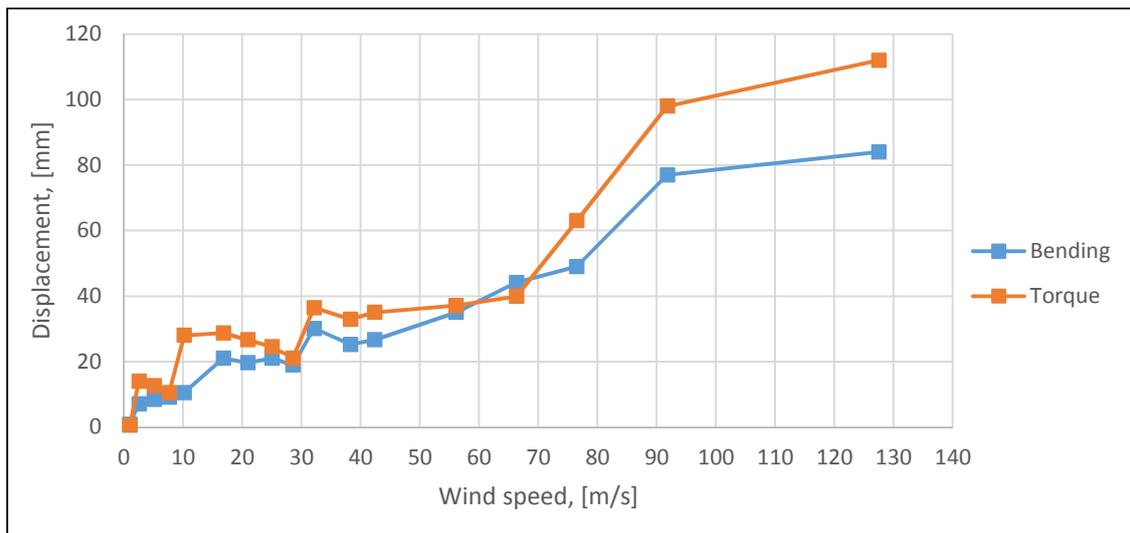
**Figure 4.** Dependence of the oscillation amplitude of the span structure of the bridge on wind speed, flow direction  $\alpha = +3^\circ$  (span located in the track).
