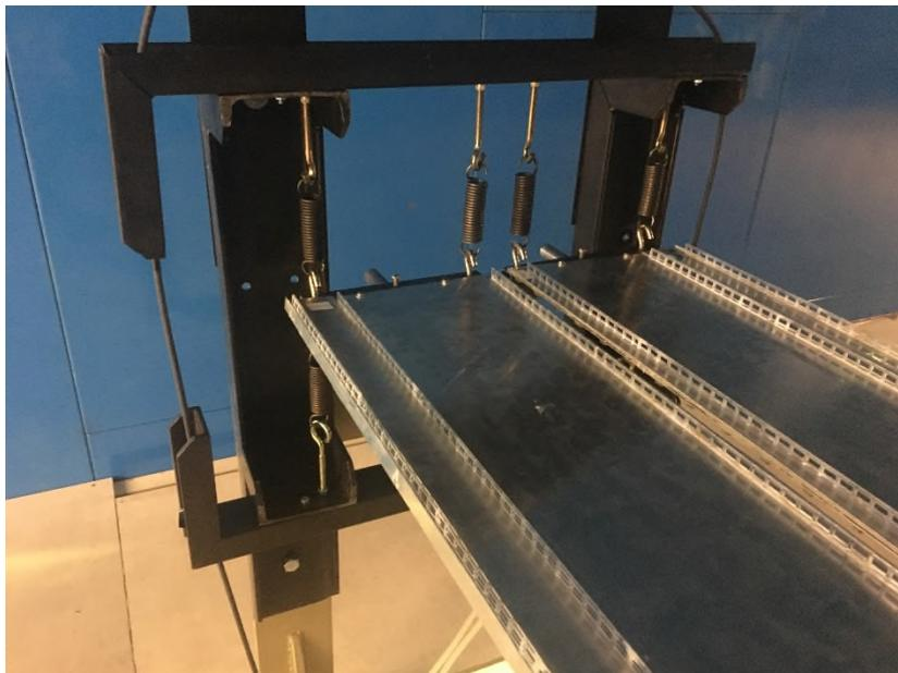
**Figure 2.** Model of a span structure on spring suspensions.
