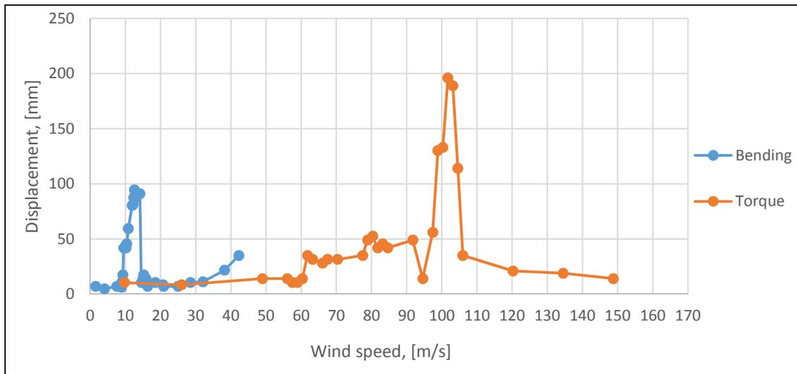
**Figure 3.** Dependence of the oscillation amplitude of the span structure of the bridge on wind speed, flow direction  $\alpha = +3^\circ$  (span on the side of the oncoming stream).
