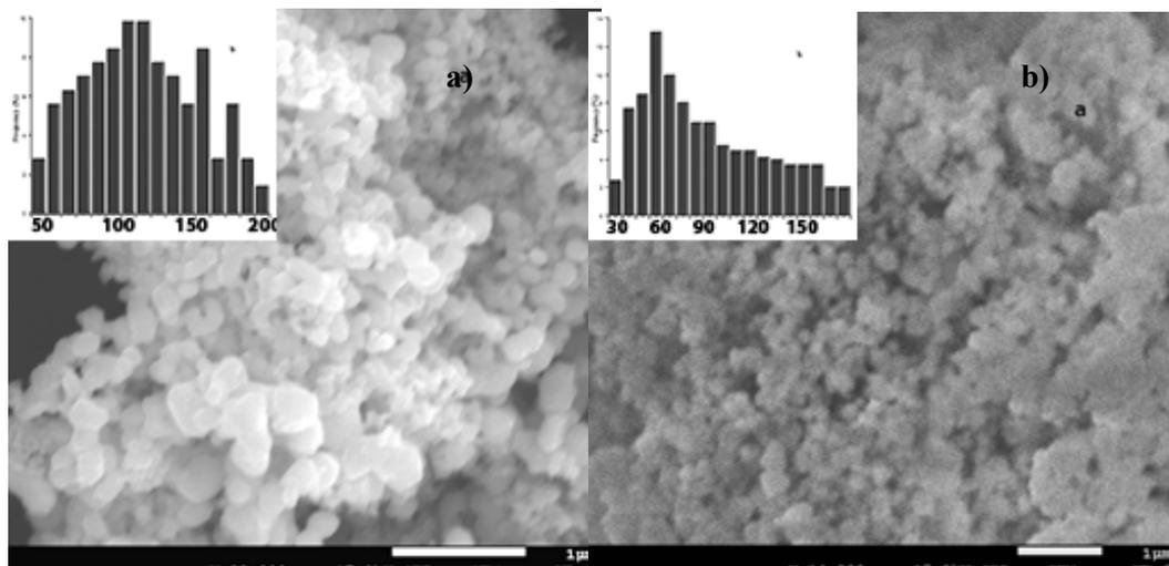
**Figure 4.** SEM images of Cu nanopowders obtained in an ammonia medium (a) and Cu nanoparticles obtained in the presence of gelatin in an ammonia medium (b) with their particle size histograms in their insets.
