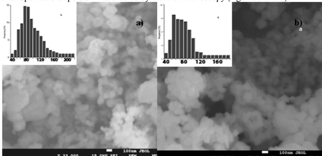
**Figure 3.** SEM images of Cu nanopowders produced in an alkaline medium (a) and Cu nanopowders obtained in an alkaline medium in the presence of gelatin (b) with their particle size histograms in their insets.
