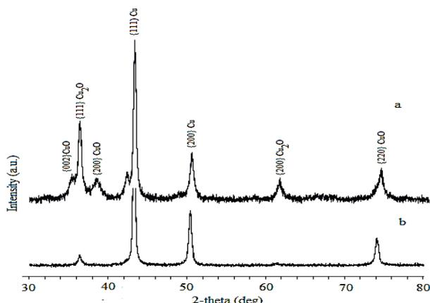
**Figure 1.** XRD patterns of Cu reduction with hydrazine products, in alkaline (a) and ammonia (b) media.
