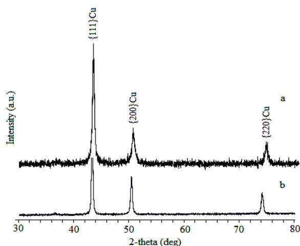
**Figure 2.** XRD patterns of Cu reduction with hydrazine products in the presence of gelatin in alkaline (a) and ammonia (b) media.
