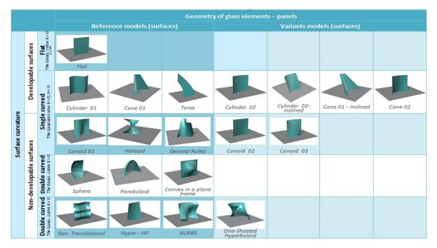
Figure 1. Typology of the glass elements according to geometry and type of curvature [1].
