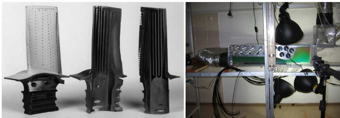
Figure 11. gas turbine blades with cooling holes (left) and view of test section for model turbine blade cooling (right)
