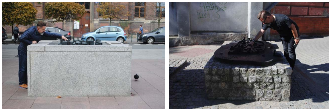
Figure 2. Problems related to construction of the pedestal, a) Poland, Kraków, too high plinth of the model, b) Poland, Chełmża, too low plinth of the model
