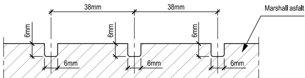
**Figure 3.** Detail of the grooving dimensions.
