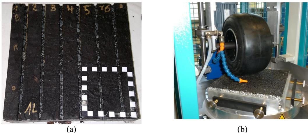
**Figure 4.** (a) Grooved plate of 26 x 26 x 5 cm used for raveling tests (b) Darmstadt Scuffing Device @ BRRC, adapted from [7].
