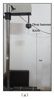
Figure 1. Stab resistance test platform.
