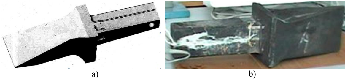
Figure 1. Bucket wheel excavator tooth: a) The tooth with the places where the strain gage will be placed, b) The tooth with soldered strain gage.
