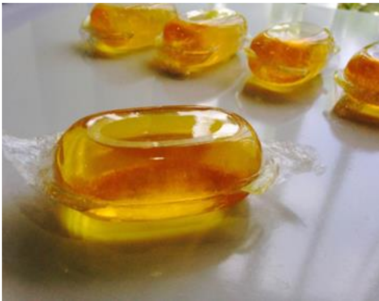
Figure 2: Premium transparent toilet soap after stamping method with stretch wrap
