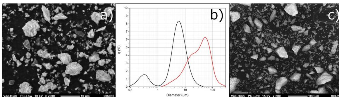
**Figure 1.** SEM images of calcined shale (a), particle size distribution (b) – black (CS) and red (filler) and SEM image of filler (c)
