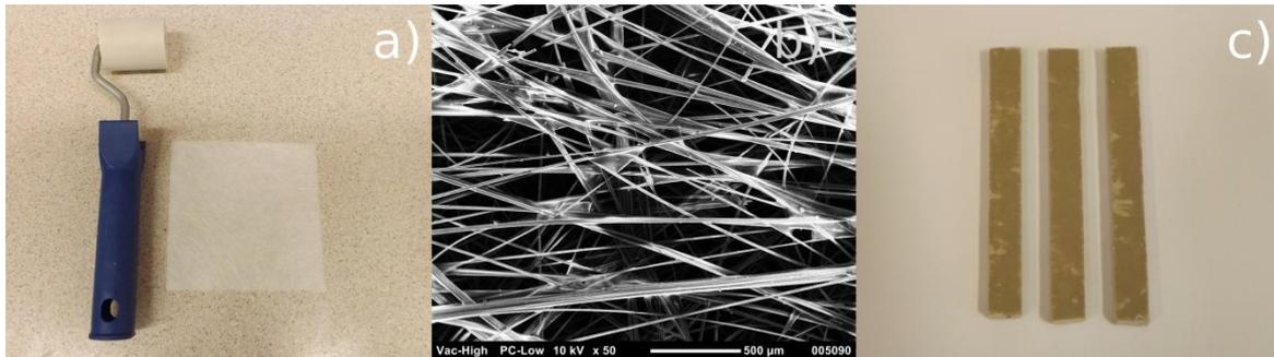
**Figure 2.** Image of hand roller and non-woven fabric (a), SEM of non-woven glass fabric (b), tested specimens (c)
