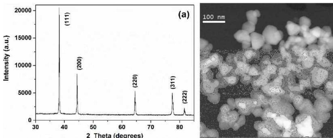
**Figure 1.** (a) XRD pattern of Ag metal nanoparticles, (b) STEM image overview of Ag MNP
