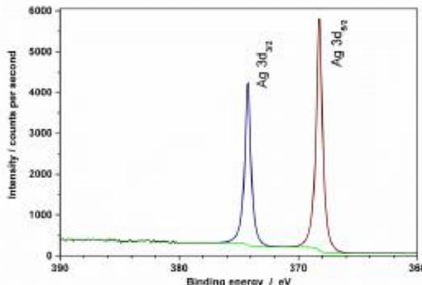
**Figure 3.** XPS spectra obtain on Ag NPs
