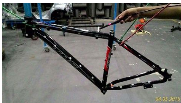
Figure 3. Impact test for EMA
