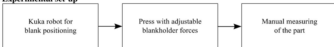
**Figure 4.** Scheme of experimental set-up
