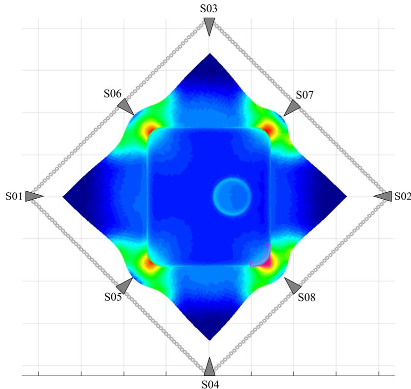
**Figure 2.** Position of virtual draw-in sensors
