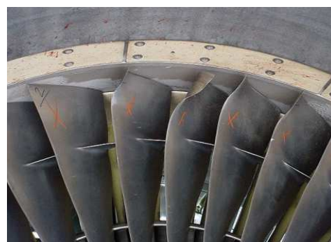
Figure 5. Engine blade damage due to an ingestion of a small bird [9]
