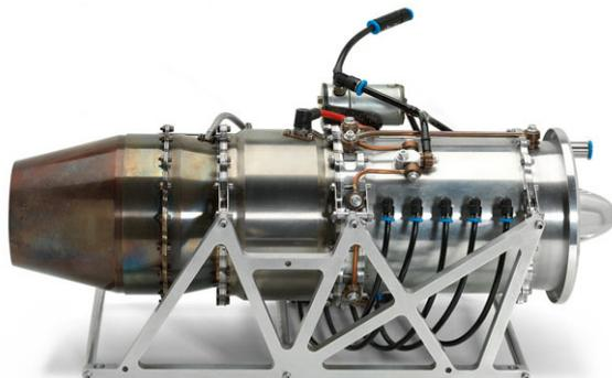
**Figure 2.** Turbojet MTE with 5-stage axial compressor and axial turbine made by Bladon firm [4].
