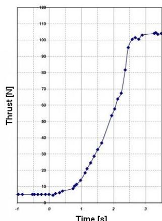
**Figure 19.** Hawk 100R turbojet engine transient performance – “spool time” [19].
