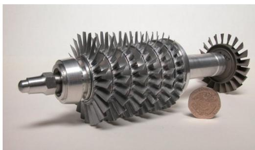
**Figure 3.** Example of the turbojet MTE single shaft with 6-stage axial compressor and axial turbine [5].
