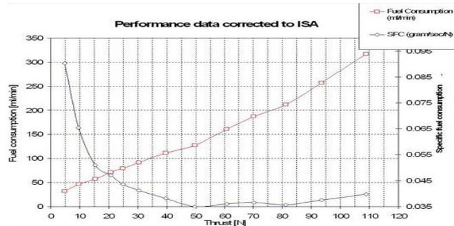
**Figure 11.** Load characteristic of Hawk 100R micro turbojet engine [13].
