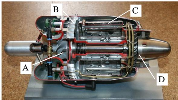
**Figure 1.** Cross section of a typical micro turbojet engine (MTE):
