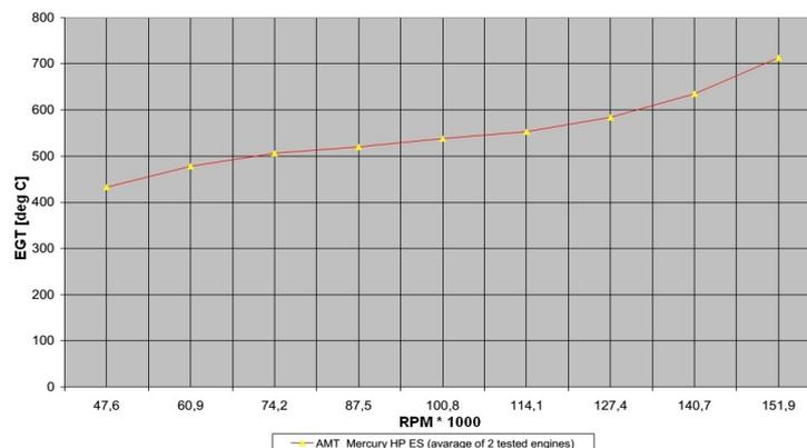
**Figure 10.** Exhaust gas Temperature (EGT) versus shaft rotational speed of AMT Mercury HP ES micro turbojet engine [11].
