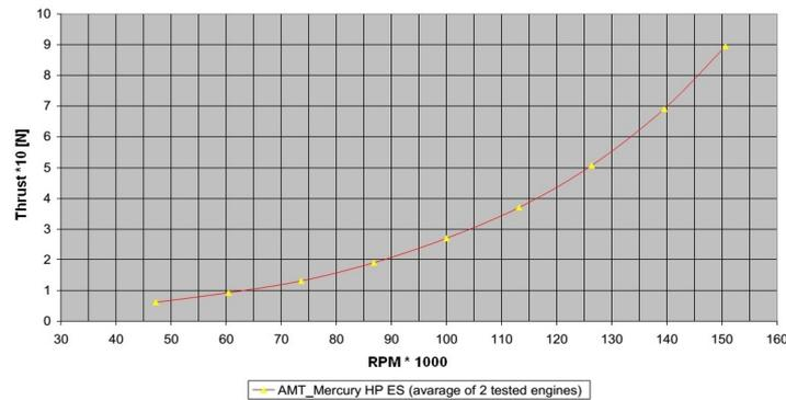
**Figure 8.** Thrust versus shaft rotational speed of AMT Mercury HP ES micro turbojet engine [11].
