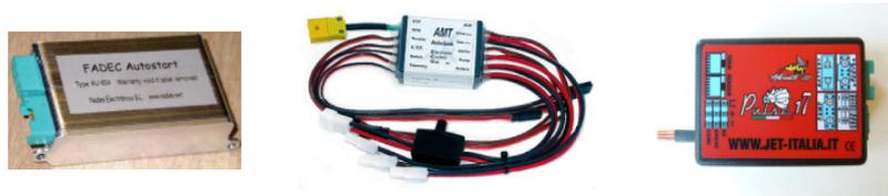
**Figure 17.** Examples of FADEC electronic control units [12, 11, 18].
