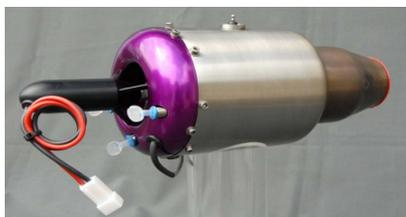
**Figure 14.** AMT Mercury HP electric start system (propane-butane or kerosene) [11].
