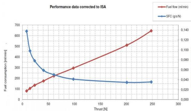
**Figure 12.** Load characteristic of Hawk 260R micro turbojet engine [14].
