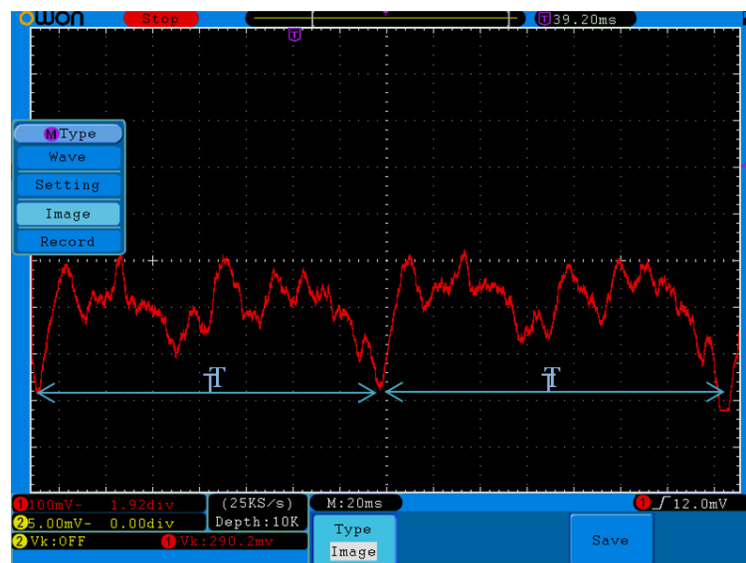
Figure 12. The screen shot from oscilloscope with shape of torque from two shaft revolutions.
