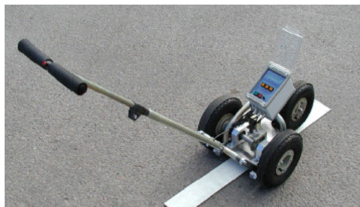
Figure 2. VTI Grip Tester.
