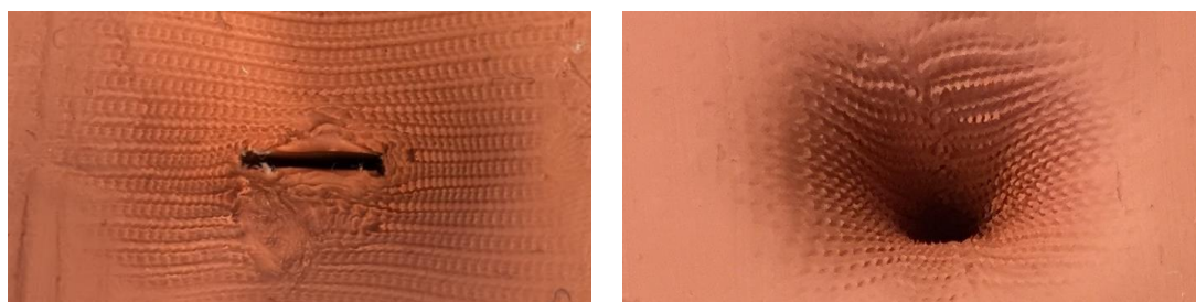
Figure 2. Cuts in plasticine, left panel: p-aramid as tested fabric, right panel: PBO as tested fabric.
