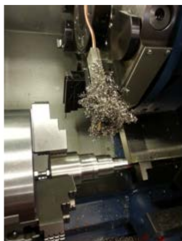
Figure 9. MQL cooling encouraging poor chip breaking at higher cutting speed.
