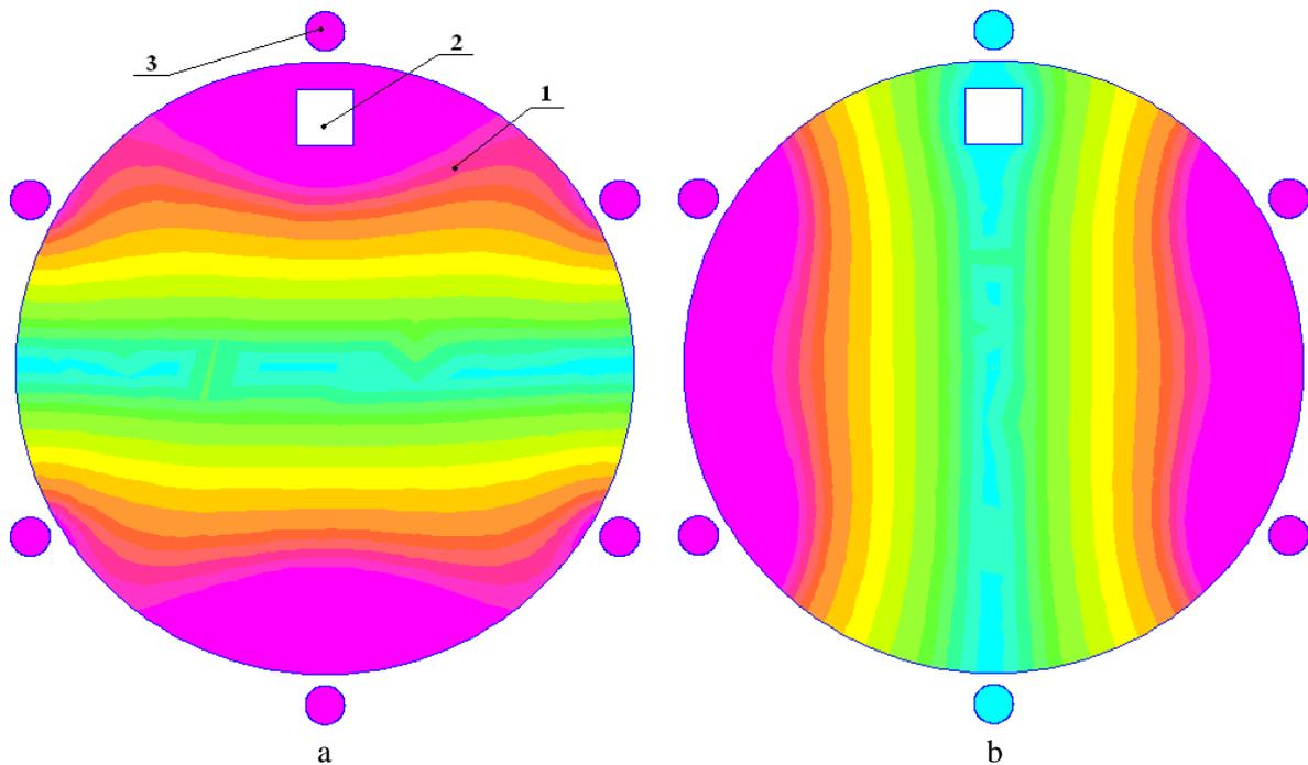
**Figure 2.** Current density distribution in a transverse section of an electrode with a frequency of 8 Hz: a) vertical current density distribution; b) horizontal current density distribution. 1 – graphite rod; 2 – place of defect; 3 – metal rod for current displacement.
