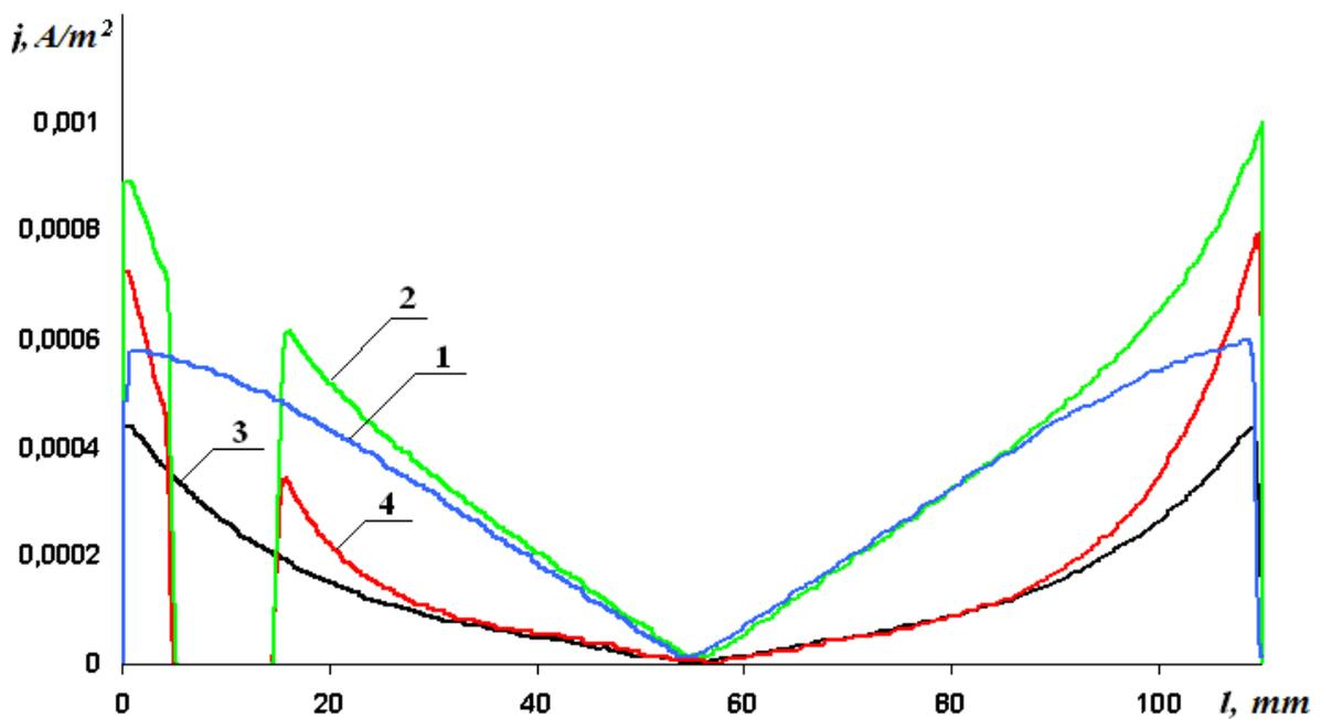
**Figure 3.** The diagram of current density distribution in a graphitized electrode: 1 – with a frequency of 8 Hz and horizontal current density distribution; 2 – with a frequency of 8 Hz and vertical current density distribution; 3 - with a frequency of 80 Hz and horizontal current density distribution; 4 - with a frequency of 80 Hz and vertical current density distribution.
