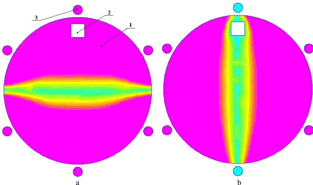
**Figure 4.** Current density distribution in a transverse section of an electrode with a frequency of 80 Hz: a) vertical current density distribution; b) horizontal current density distribution. 1 – graphite rod; 2 – place of defect; 3 – metal rod for current displacement
