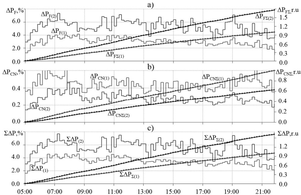
**Figure 4.** Daily average curves of relative power loss: a – in feeders; b – in CN; c – total.
