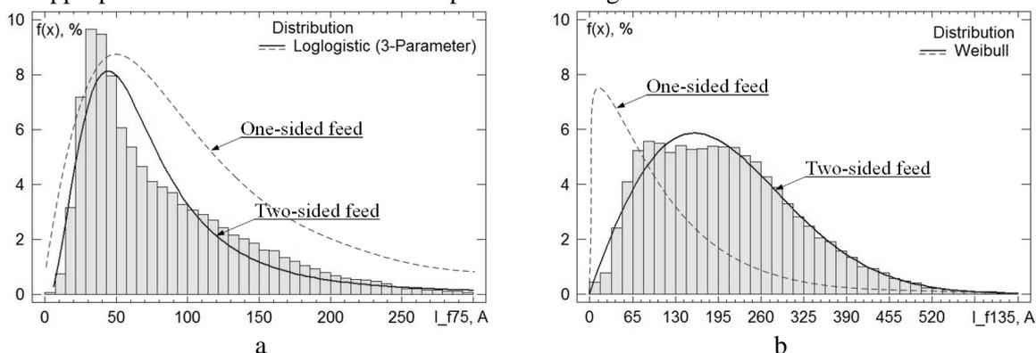
**Figure 2.** The statistical distribution functions of feeders currents
