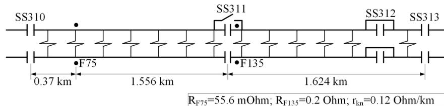
**Figure 1.** The supply and sectioning circuit of investigated TN area
