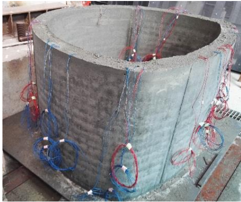
Fig.1 Test model of full section tunnel
