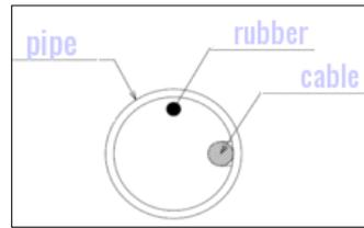
**Figure 2.** Detail of cable clamp inside the pipe.
