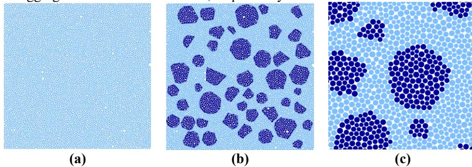
**Figure 2.** Numerical model: (a) The initial fine particle system; (b) The particle system with coarse aggregate; (c) The details view of model. The dark blue particles denote coarse aggregate, while the light blue particles denote cement.
