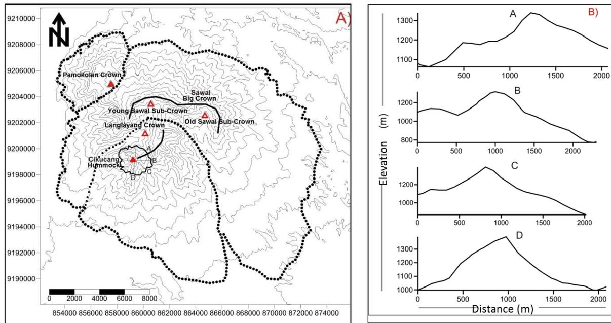
**Figure 11.** (A) Topographic map with cross section line in Cikucang Hummock. (B) Distance vs elevation profile of Cikucang Hummock which shows a relatively conical shape.
