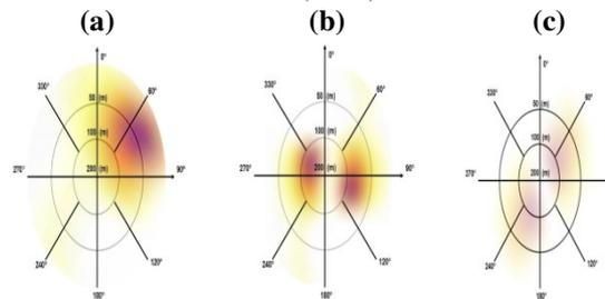
**Figure 2.** Ocean wave spectra derived from (a) AWAC, (b) ENVISAT ASAR and (c) velocity bunching model.
