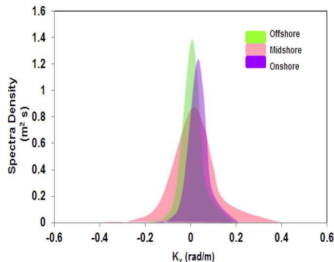
**Figure 3.** Wave spectra energy simulated from the velocity bunching algorithm.
