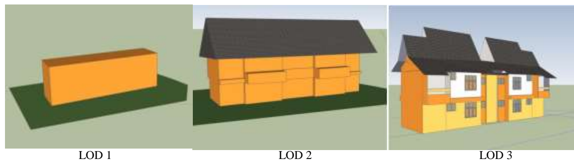
Figure 9. Resulted model in LOD 1, LOD 2, and LOD 3.
