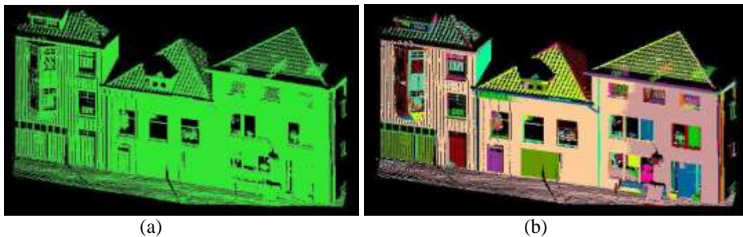
Figure 2. (a) point cloud before segmentation (b) point cloud after segmentation process.
