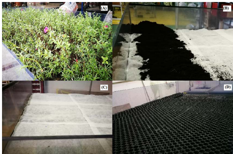
Fig. 1. Experimental green roof test beds that established in this study.
