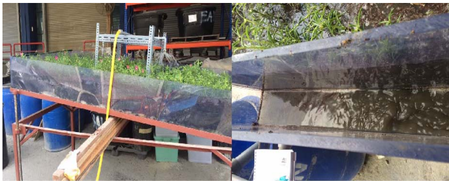
Fig. 2. Simulated rainfall (a) and measurement of flow rate (b) during the experiment.
