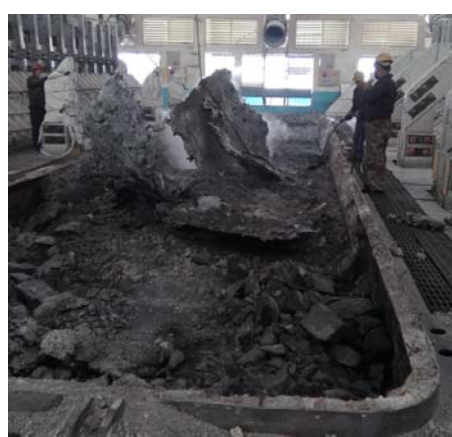
Fig. 2 Overhaul slags of the electrolytic cell
