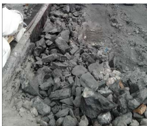
Fig.1 Electrolytic cell spent lining
