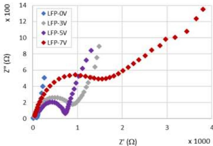
**Figure 4.** Cole-Cole plots of EIS test results for 0 wt.% V-doped, 3 wt.% V-doped, 5 wt.% V-doped, and 7 wt.% V-doped LiFePO<sub>4</sub>/C
