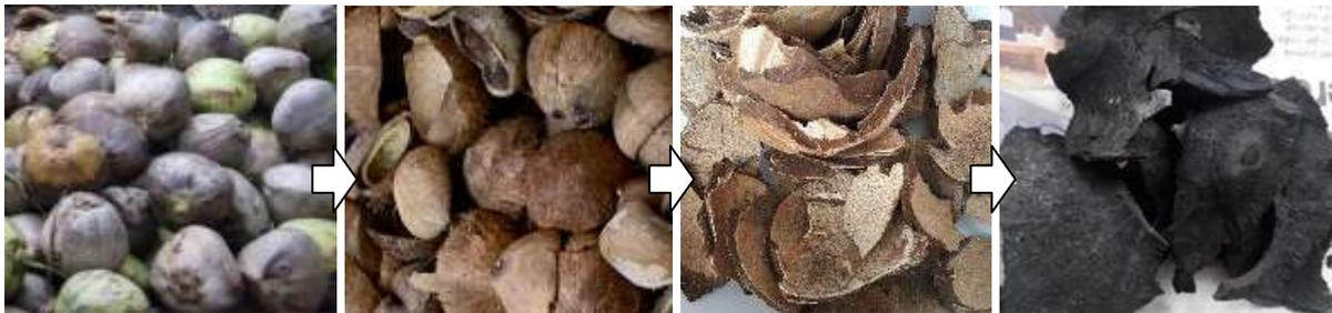
**Figure 1.** Steps in carbon pyrolysis from coconut shell. Left to right is coconut, coconut shells, chopped and dried coconut shells, and coconut shells after pyrolysis.
