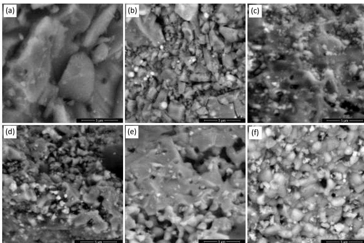
**Figure 3.** Secondary electron images of (a) activated carbon from the coconut shell; (b) as-synthesized  $\text{LiFePO}_4$ ; (c) 0 wt.% V-doped  $\text{LiFePO}_4/\text{C}$ ; (d) 3 wt.% V-doped  $\text{LiFePO}_4/\text{C}$ ; (e) 5 wt.% V-doped  $\text{LiFePO}_4/\text{C}$ ; and (f) 7 wt.% V-doped  $\text{LiFePO}_4/\text{C}$ . The bar scale is 5  $\mu\text{m}$ .
