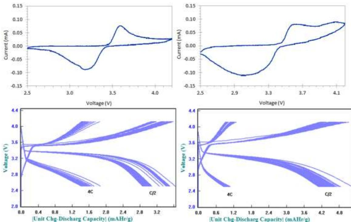
**Figure 5.** Cyclic voltammetry (top) and charge/discharge (bottom) curves for the LiFePO<sub>4</sub>/V/C at 3 wt.% V (left) and 7 wt.% V (right)
