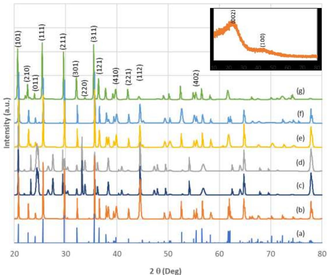
**Figure 2.** Diffraction patterns of (a) reference  $\text{LiFePO}_4$ , (b) commercial  $\text{LiFePO}_4$ , (c) as-synthesized  $\text{LiFePO}_4$ , (d)  $\text{LiFePO}_4/\text{C}$  at 0 wt.% V, (e)  $\text{LiFePO}_4/\text{C}$  at 3 wt.% V, (f)  $\text{LiFePO}_4/\text{C}$  at 5 wt.% V, and (g)  $\text{LiFePO}_4/\text{C}$  at 5 wt.% V. Inset is the X-ray diffraction pattern of the activated carbon from the coconut shell
