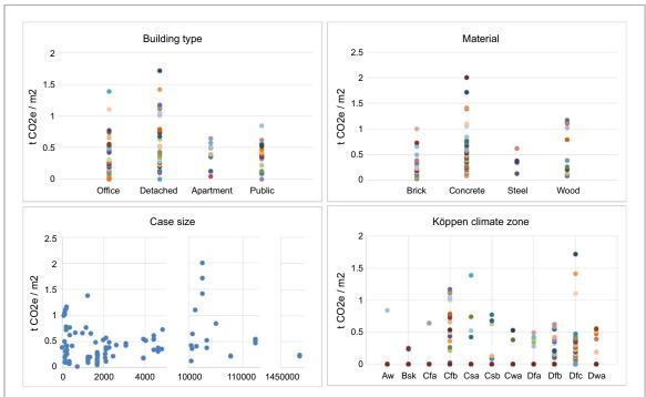
Figure 2. The results of the 116 case studies according to the building types, materials, sizes, and climate zones showing the wide variation even within similar classes of buildings.
