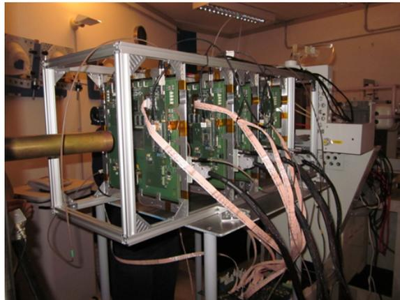
**Figure 2.** picture of the PRIMA/RDH pCT scanner mounted at the CATANA beam line.
